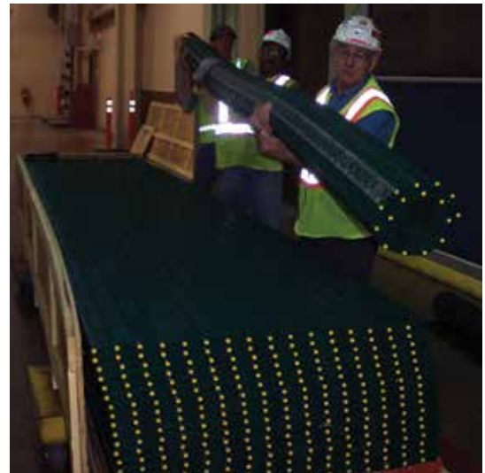
Chain is Coiled and Properly Supported
